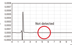
Sample carryover test using Chlor-hexidine
